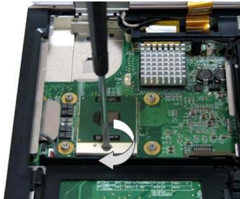
Fig. 19 Releasing the CPU lock
